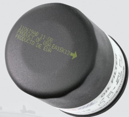
▲ AMSOIL Oil Filters feature a reference arrow to aid in proper installation. Once the filter is finger tight, it is easy to gauge the additional three-fourths to 1.25 turns required to ensure a good fit. Over-tightening can lead to leakage.
